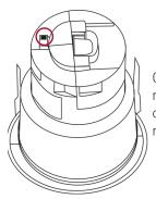
Carefully remove the metal locking clip, circled left, from rear of unit.
