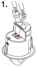
Connect the DALI terminal blocks. If required, connect the external power cable.
