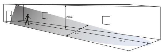
Detector head position at 80° to the vertical for large offices or classrooms, and for corridor and aisles. Sensitivity set to maximum.
