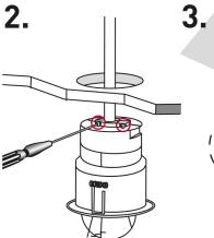
Attach the cable clamp.
