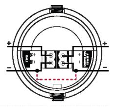
link between the DALI negative terminal and the negative terminal of the external power supply, as shown in the figure.
